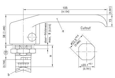
Installed position of the housing, seen from outside of the door, at
